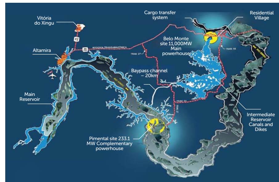
Main distances: from Altamira to Belo Monte Site: 55 km. From Altamira to Pimental Site: 65 km. From Vila Belo Monte Residential to Belo Monte Site: 6 km. From Belo Monte Residential Village to Pimental Site: 49 km.
